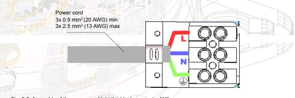
Fig. 3.3. Assembly of the power cord into the block connector [11]
