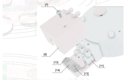
Fig. 3.2: Disassembly of the terminal cover
